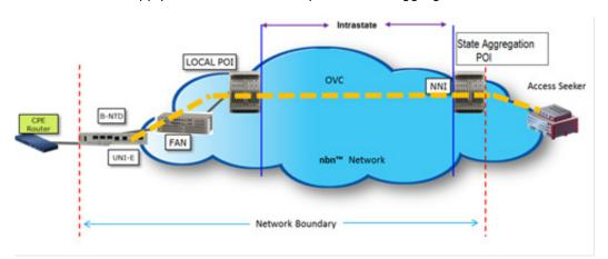
(b) The diagram below depicts an example of **nbn**® Enterprise Ethernet as one part of the overall network supply chain where RSP does not acquire Route Aggregation:
