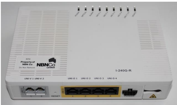
Figure 9. Stand-alone NTD Modules – Indoor and Outdoor
