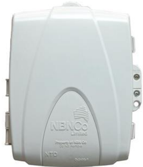
Figure 9. Stand-alone NTD Modules – Indoor and Outdoor
